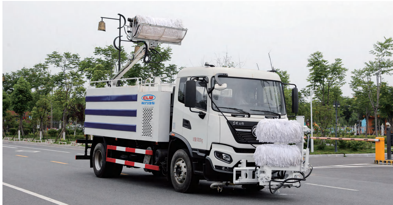
Dongfeng KR Tunnel Guardrail Cleaning Truck
